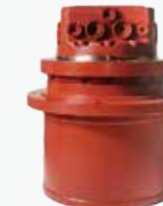
TM04I 3-4T excavator For SK40/Bobcat 331D 425 Kubota KX101/U30/KX91.2 IHI Imer 25J Volvo/EC30 CX36/YC35
